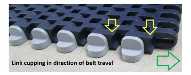
NOTE: The two sides of the belt have a slightly different link edge profile, one is concave and one is square, ensure the same profile matches on either side when joining the belt sections.
