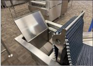
**3.** Lift the hinge to release the tension on the belt.
