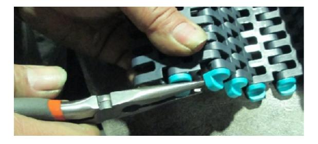
2.8.3 When joining the belt sections ensure the link orientation matches (see photos below on the two link profiles on either side of the belt):
