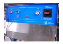
2. Loosen the screws on the dial and pull the dial off.
