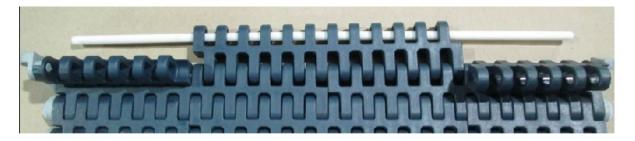
2.8.2 The tabs on either side hold the pin in place, they are installed or removed by twisting them gently using pliers:
