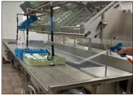
2. Start spraying along the belt from right to left, beginning at the entrance and continuing all the way to the end. Ensure all food is washed off the belt.
