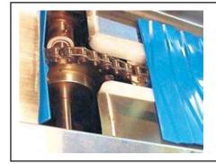
Jog the belt where slats are to be replaced to top of the bed or on the drive sprocket just before entering the belt slot.
