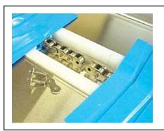
Remove required number of links. Removal of each outside & inside link pair reduces the overall chain length by 1 ½".
