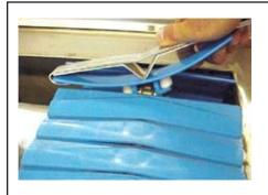
Arch the slat using the slat tool and engage the chain pins on one side. Push the arched slat to the chain with a rolling motion to the opposite side.
