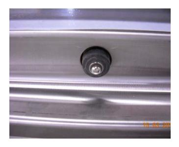
Note: When washing the conveyor never direct the hose spray towards the accumulation switch. If water gets into the switch it will malfunction. The accumulation switch prevents jamming of trays and if it malfunctions it must be replaced immediate.
