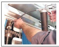
Lubricate the bearing using a grease pump.
