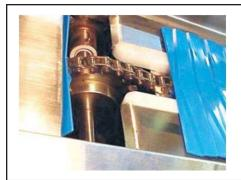
Remove a few slats to access the grease nipples.
