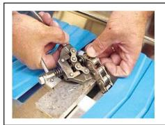
Overlap the chain to determine where the next slat link should be disassembled & re-connected.
