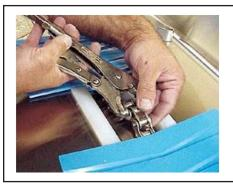
Re-connect the chain by press-fitting the side link onto the pin link. (Channel-Lock or Vice-Grip pliers work well).
