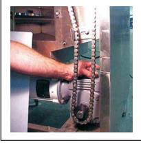
Take out the socket headed screw located at the bottom to drain the oil from the gearbox.
