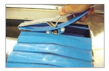
**Note:** The slat tool aides in removal & installation of slat and is available for purchase from Aerowerks.
